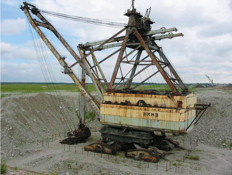
Fig. 4. Largest in Europe bucket excavator EVG35/65 with bucket holding capacity of 35 m 3 and weighing 4021 t in the Aidu opencast. Photo by Ingo Valgma.
