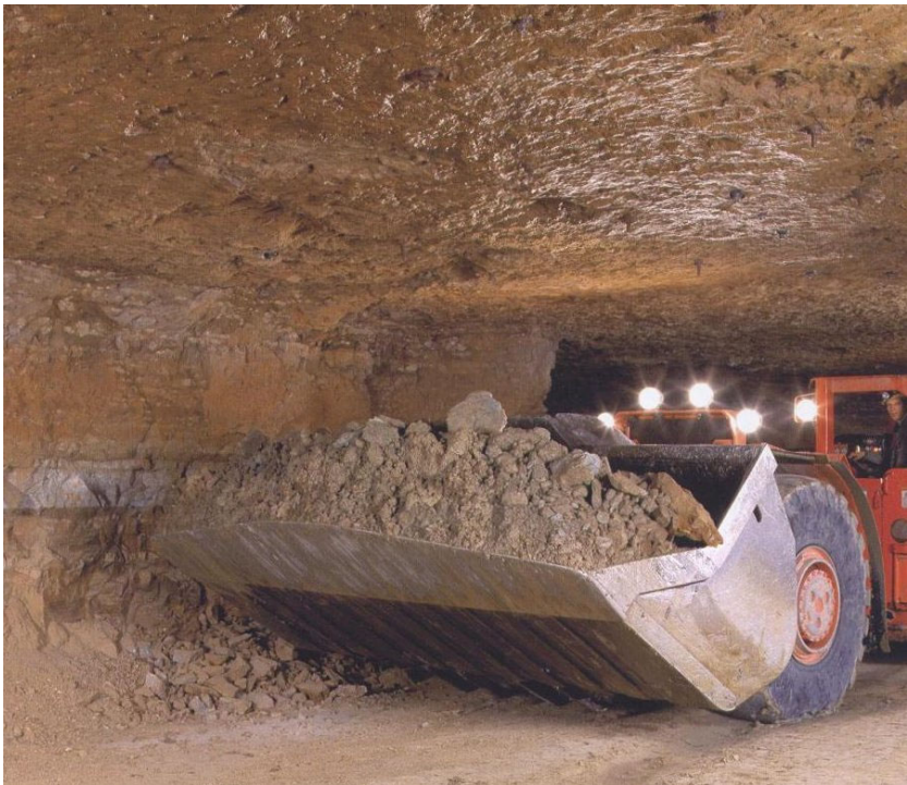
Fig. 3. In pillar mining, the roof and the mined-out land are supported with pillars of unextracted rock, with some 25% losses of oil shale. Photo by Heikki Bauert.
